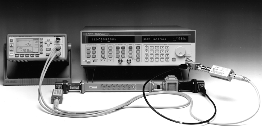
Figure 5-10. E4419B dual-channel power meter measures insertion loss of a 11.245 GHz waveguide bandpass filter, using its power ratio mode, plus a sweeper and power splitter. Agilent’s 90-dB dynamic-range sensors are ideal for such high-attenuation measurements.
